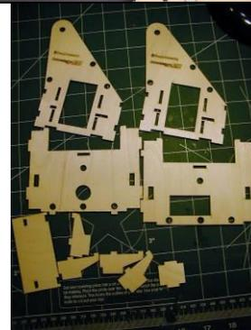
Lay the side supports as shown, and install the small reinforcement pieces.
