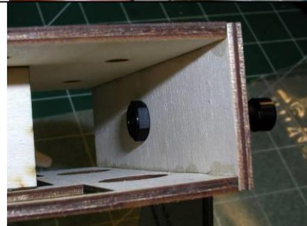
With the servo centered, align the antenna support to the line shown (no line on beta models, align at a 45 degree angle from vertical). Attach servo to servo horn on the side support.
