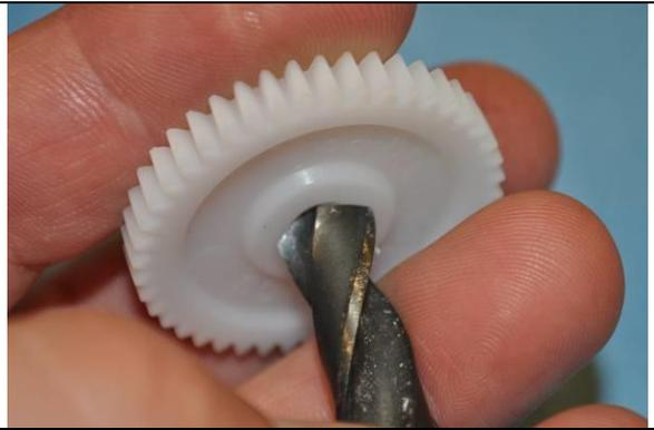
Mist the servo arm with kicker, and apply some CA to the gear as shown. This will hold the gear in place for drilling screw holes. Carefully (and quickly!) place the servo arm on the gear, making sure it's centered as perfectly as possible.
