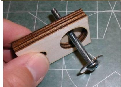
On the opposite side, add a washer and a nut. Tighten securely.
