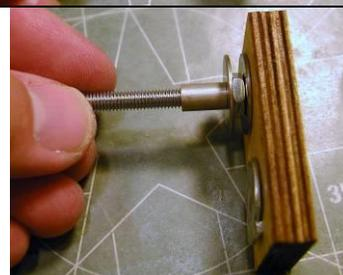
With a hobby knife, scrape a small amount of material from the holes on the top and bottom plates until the threaded spacer slides through without binding. Do not remove too much material or there will be excess slop in the pan assembly.
