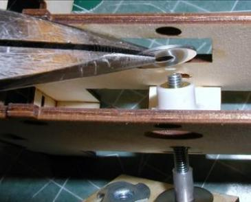
Insert the bolt through the hole on the top plate, and add the second threaded spacer.
