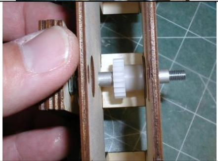
Add the last washer and the nut to the bolt and tighten securely. A good amount of force is helpful to prevent any slippage of the assembly during use. At this time you should also tighten the set screw on the gear.
