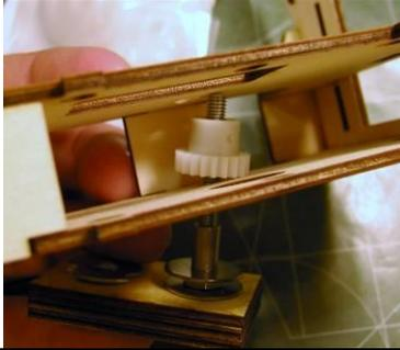
Using needle-nosed pliers, add a washer above the gear.
