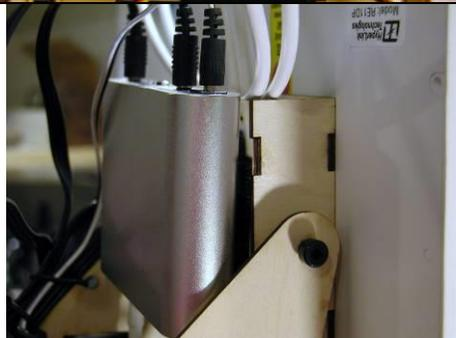
The EzOSD is mounted to the back plate using the hook and loop tape.
