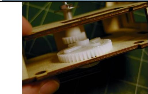
After adding the spacers included with the servos, place the servo in the hole as shown and push the gear assembly onto the servo shaft. Making sure the servo gear is engaging the smaller gear snugly, screw the servo into place using the included screws.
