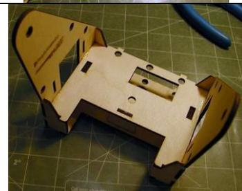
Obtain the three pieces for the tripod mount shown. The medium sized holes in the bottom of each part will all be aligned during the assembly in the next step.
