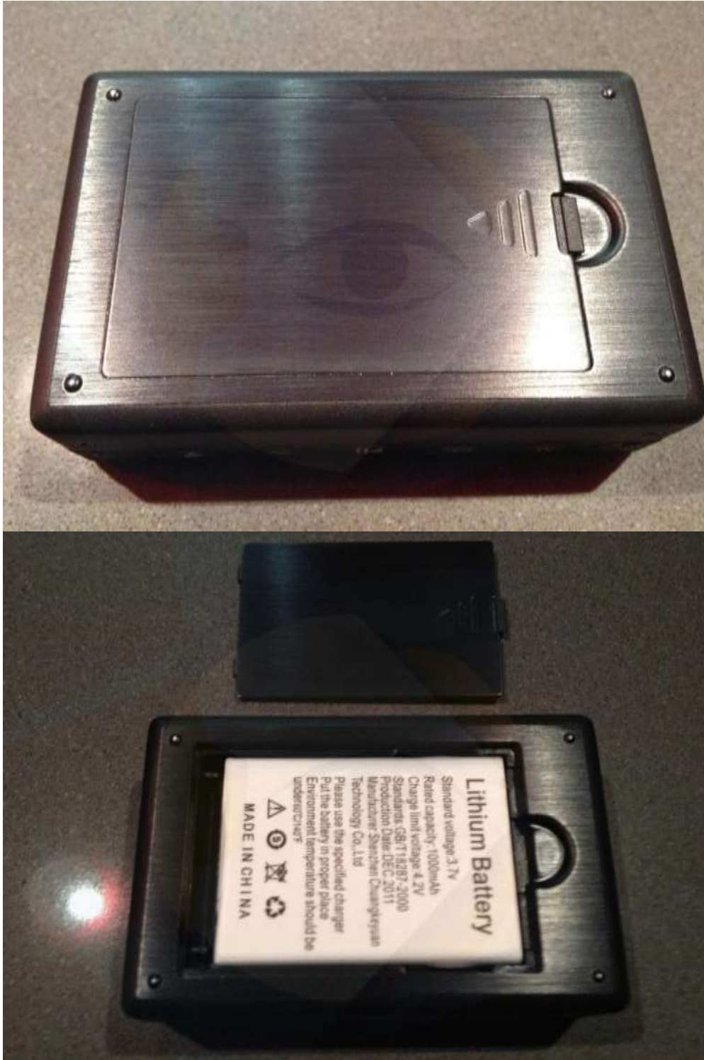
a) "Battery Door" – Reveals the internal battery
