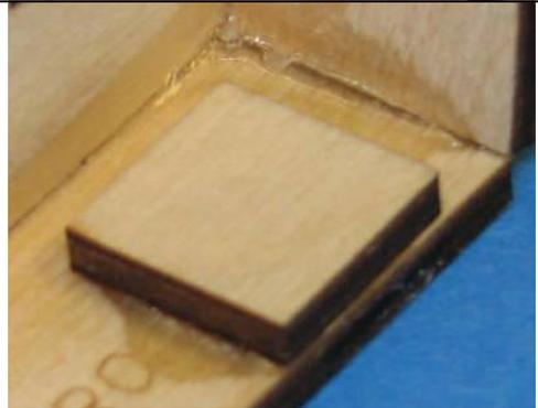
5. Install the pan/tilt mounting platform pieces as shown.
