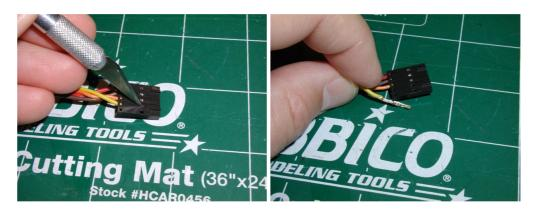
Then, gently bend the clip back up as shown, and insert the connector into the outside slot. You're done!
